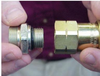
Lightly lubricate the O-Ring on the adapter and thread it into the coupling. Hand-tighten, ensuring that the O-Ring is not pinched during installation.
