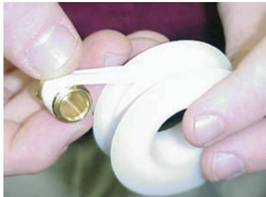
Apply 1½ to 2 wraps of PTFE tape, starting one or two threads from the lead edge, in a clockwise direction. For 316 stainless steel, be sure to use stainless grade tape.
