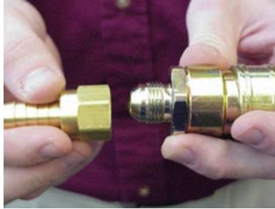
Lightly lubricate the flare on the adapter and thread it into the coupling. Hand-tighten, ensuring that the flare is seated correctly during installation.
