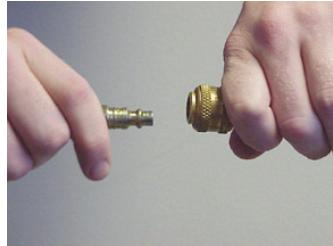
After the line is fully exhausted, you are able to safely separate the nipple from the coupler.
