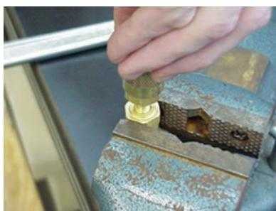
Apply lubricant sparingly to the reusable barb before inserting it into the ferrule.
