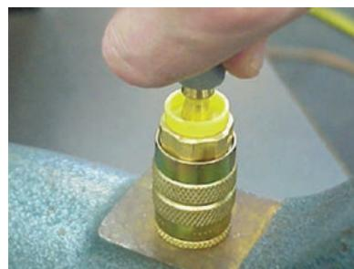
Place the end of the fitting against a flat object and grip the hose one inch from end. Push with a steady force until the end of hose is covered by the yellow plastic cap.
