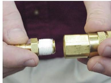
Check threads to make sure there is no obvious damage on either half and that tape is properly installed. Align male and female threaded connections and carefully begin threading the two halves together.
