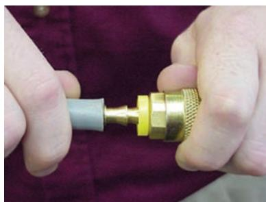
Trim hose end squarely and lubricate the Push-Loc barb and hose. Insert Push-Loc barb into the hose until first barb is inside the hose.
