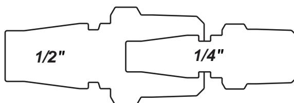
**!** Operating pressure for couplings utilizing hose barb end connections may be dramatically reduced to that of the hose rating and/or hose end connection combination. Consult hose manufacturer's catalog for hose end connection ratings. If in doubt, test under controlled conditions for suitability to application. Dixon Quick Coupling cannot assume liability for misapplication of production resulting in equipment down-time, lost production, and/or personal injury including death.
