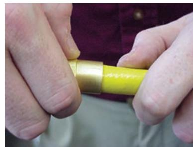
Install ferrule by slipping it onto the end of the hose and twisting it counter-clockwise.
