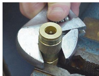
Turn the reusable fitting into the ferrule until coupling is seated against ferrule.
