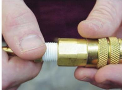
Finger tighten the connection and create a reference mark on the hex of the hose end/adapter and the coupling. This mark will help identify the number of revolutions during the next step in the procedure.
